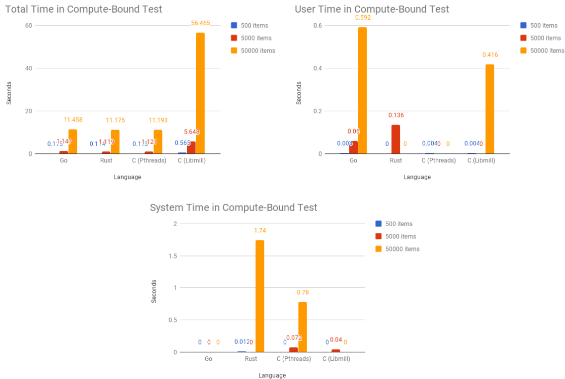
Fig. 2. For each producer-consumer implementation, we measured the total, user, and system time spent in a simulated compute-bound workload.
